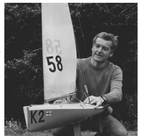
1978 significant rigs: Mark 1 soon discarded kicking strap as unnecessary and jib horse, which couldn't properly control leech tension variation. The jib boom offset pivot unlocked the 'magic' of the balance of forces that still applies today!
