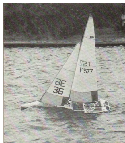
Above, the winning French boat Rajah by Pierre Jahan pictured in Race 24, Fleet A by Mike Kemp's camera. Hull is epoxy/glass/carbon fibre; carbon fibre mast and Mylar sail material.
